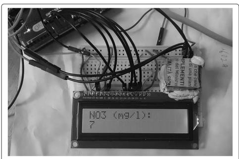
**Fig. 1** "Arduino based prototype for automatic test strip reading". A TCS3200 colour sensor in a controlled dark room is employed to read commercially available test strips. Copyright of the author
